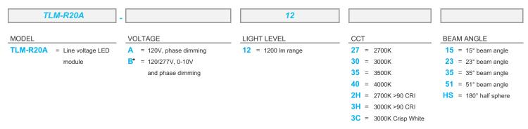
\* If connected to a phase dimmer, the pushbutton activated light output control is automatically de-activated and the dimmer will be the sole method for controling light output. If connected to a 0-10V dimmer, the lowest pushbutton setting is de-activated. See page 2 for more information on R20 pushbutton activated light output control.
